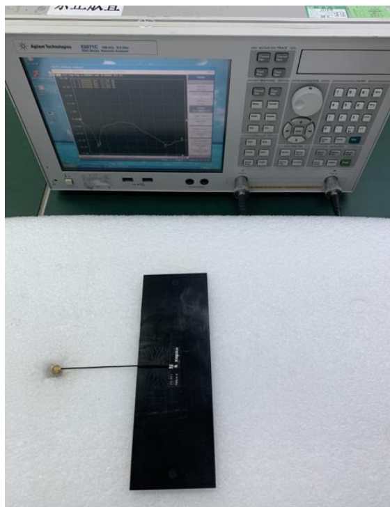
ANTENNA LOADED WITH PC/ABS BLOCK OF 1.5 MM THICKNESS WITH VNA
