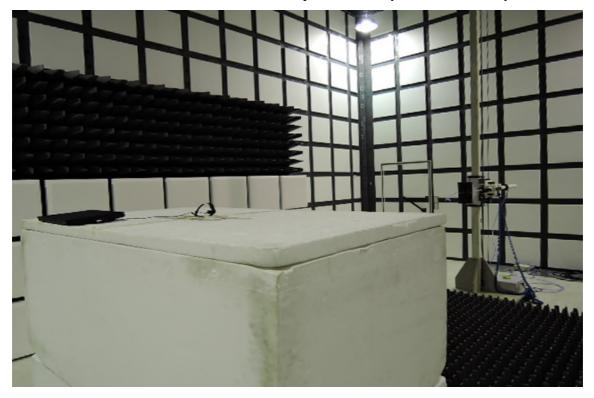
Radiated Emission Set up Photos (Front View)
