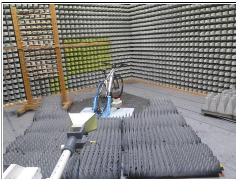
Figure 6-3: test setup for radiated disturbances 1 GHz to 2 GHz
