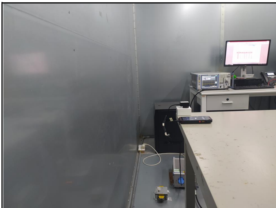
Fig. 4 Power line conducted emission setup photo
