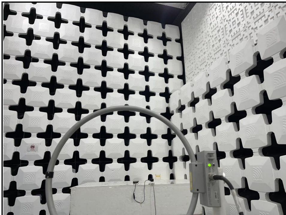
Fig. 1 Radiated emission setup photo(Below 30MHz)
