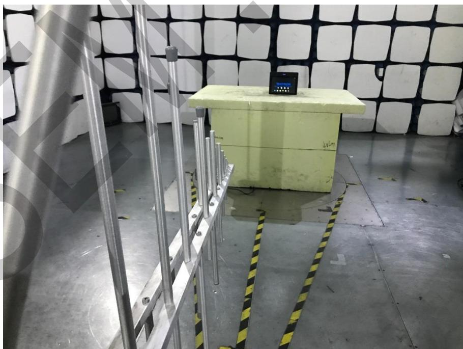
**Radiation Emission Test Setup (1GHz to 18GHz)**
