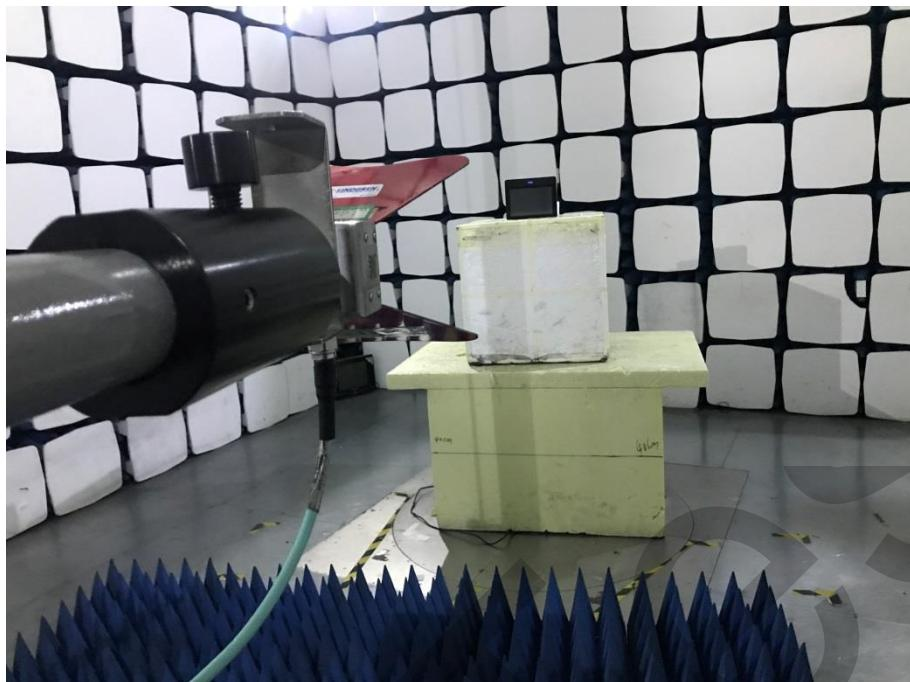
**Radiation Emission Test Setup (Above 18GHz)**
