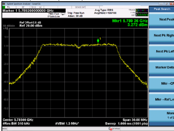
(802.11a) PSD plot on channel 157
