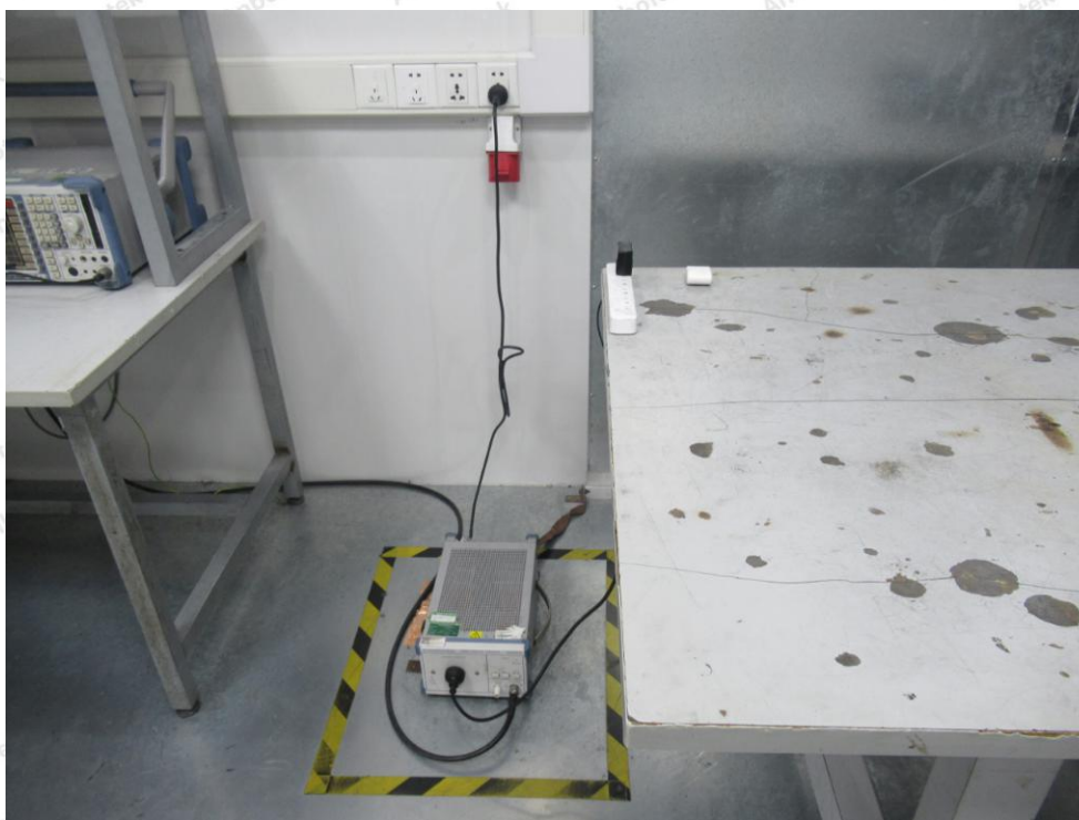
Photo of Conducted Emission Measurement
