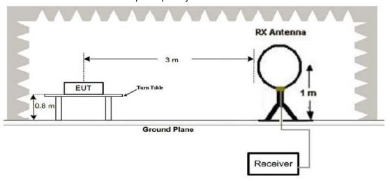
(2) Radiated Emission Test-Up Frequency 30MHz~1GHz
