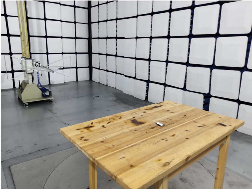
Photo of Radiated Emission Measurement
