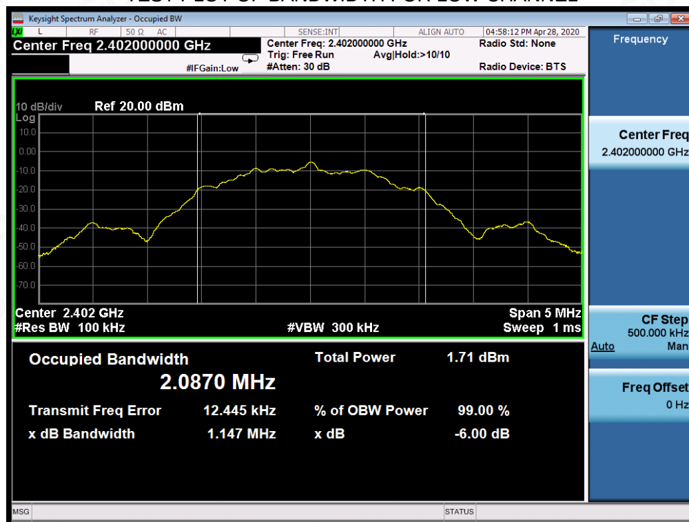
TEST PLOT OF BANDWIDTH FOR LOW CHANNEL
