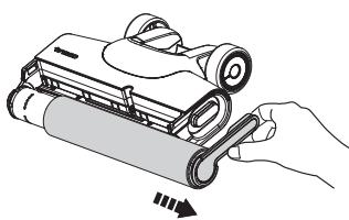
Remove the brush roller by grabbing the brush roller tab and pulling out.
