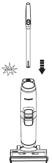
To assemble the handle, insert it into the appliance until you hear a click.
