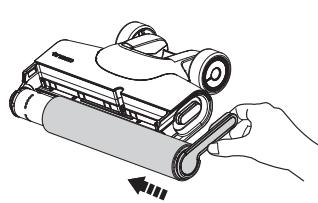
Replace the brush roller by inserting its end into the left side of the holder, then attach the roller tab to the magnetic buckle on the right side to lock into place.
