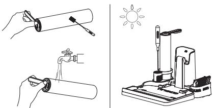
Use the cleaning tool to remove the hair and debris wrapped around the roller and then rinse the roller with water. Replace the brush roller back into the accessory holder, and allow it to dry completely before reinstalling.
