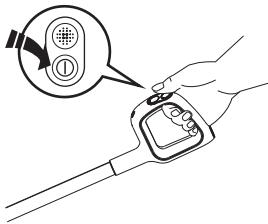
Press the ① button and the appliance will start in AUTO mode by default. Press it again to turn off the appliance. Switch between AUTO, MAX and SUCTION modes by pressing the
