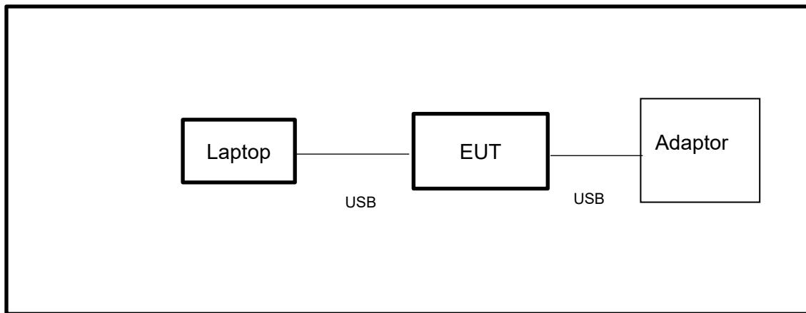
Note: Adaptor only use for AC POWER LINE CONDUCTED EMISSION test
