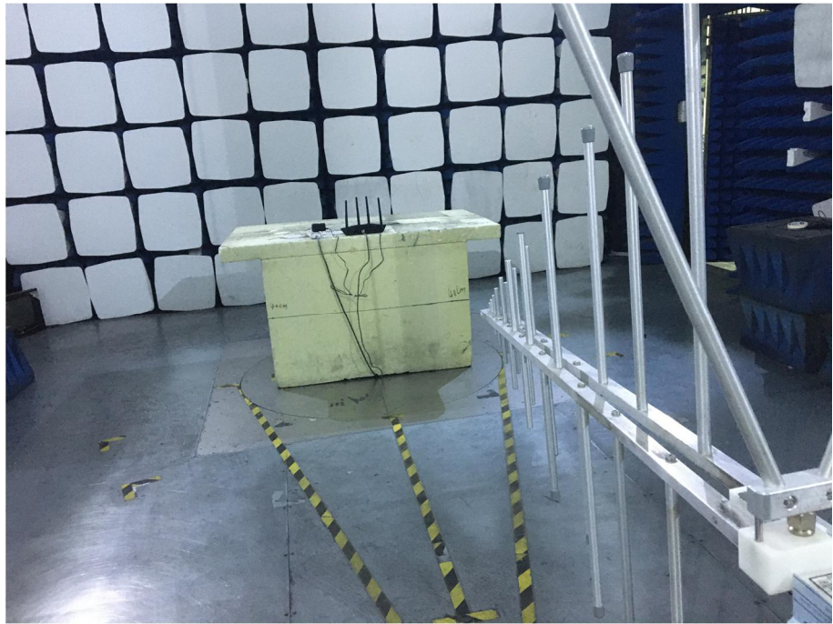
Radiation Emission Test Setup (30MHz to 1GHz)
