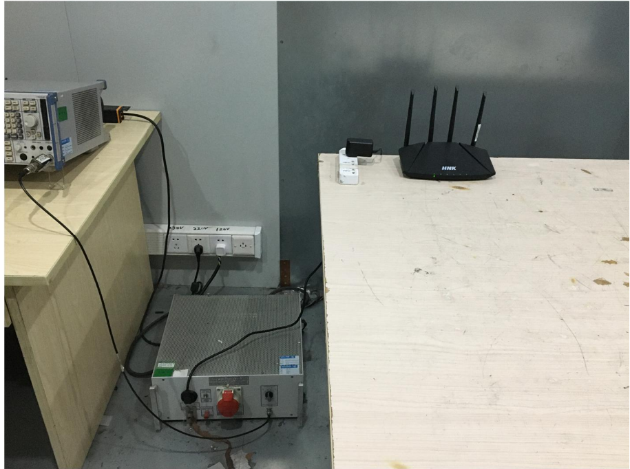
Conducted Emission Test Setup
