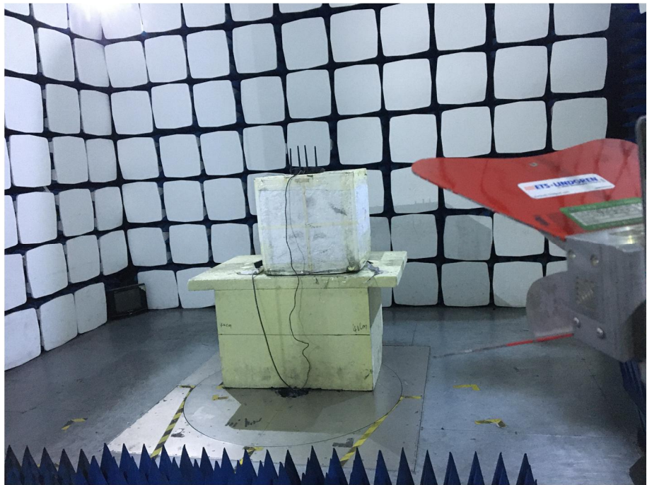
Radiation Emission Test Setup (1GHz to 18GHz)
