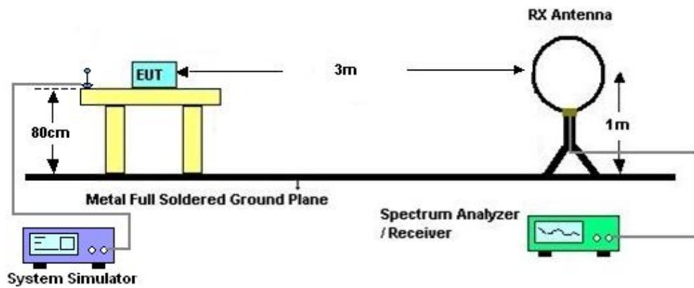
For radiated test from 30MHz to 1GHz
