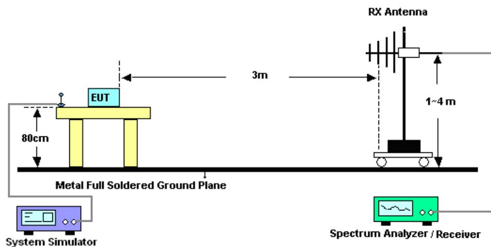
For radiated test above 1GHz
