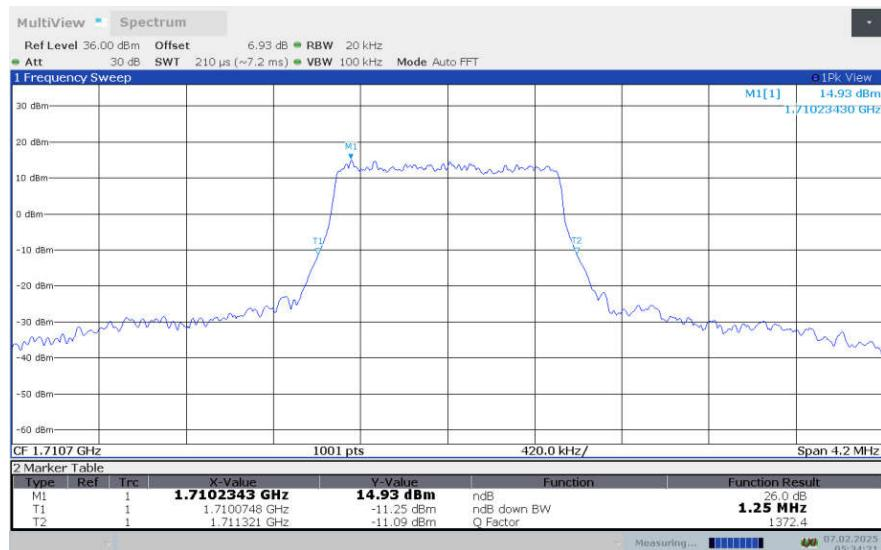
**LTE Band 4, 1.4MHz Bandwidth,LOW,64QAM (-26dBc OBW)**
