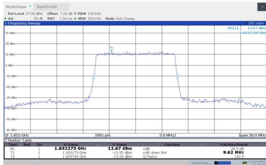
**LTE Band 2 , 10MHz Bandwidth,LOW,64QAM (-26dBc OBW)**
