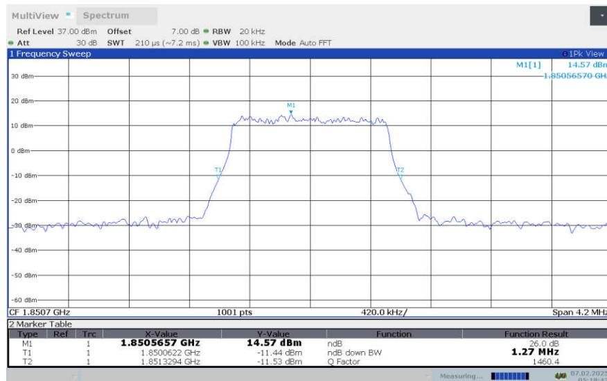
**LTE Band 2, 1.4MHz Bandwidth,LOW,64QAM (-26dBc OBW)**
