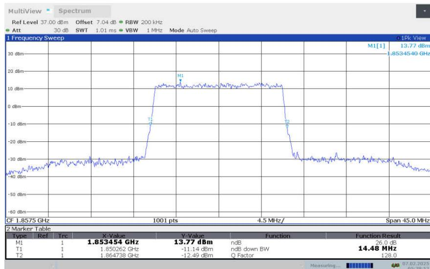
**LTE Band 2, 15MHz Bandwidth,LOW,64QAM (-26dBc OBW)**
