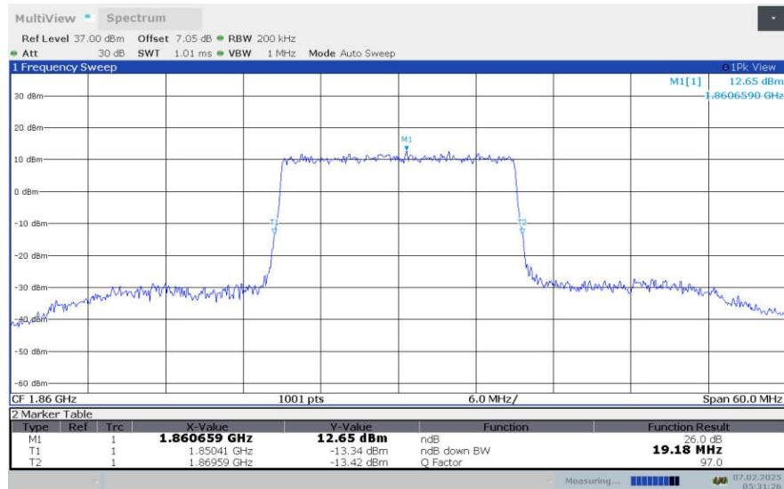
**LTE Band 2, 20MHz Bandwidth,LOW,64QAM (-26dBc OBW)**
