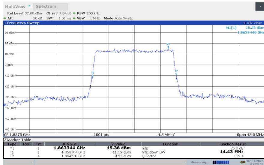
**LTE Band 2, 15MHz Bandwidth,LOW,16QAM (-26dBc OBW)**
