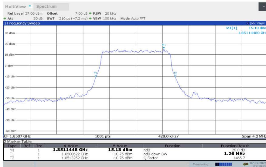
**LTE Band 2, 1.4MHz Bandwidth,LOW,16QAM (-26dBc OBW)**
