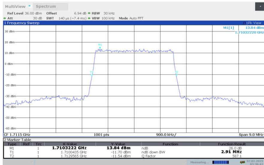
**LTE Band 4, 3MHz Bandwidth,LOW,16QAM (-26dBc OBW)**
