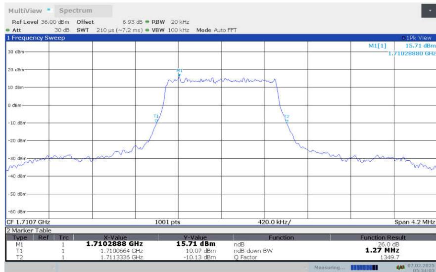
**LTE Band 4, 1.4MHz Bandwidth,LOW,16QAM (-26dBc OBW)**
