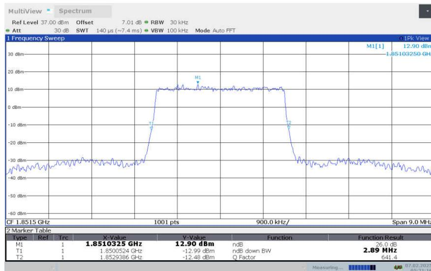
**LTE Band 2, 3MHz Bandwidth,LOW,64QAM (-26dBc OBW)**
