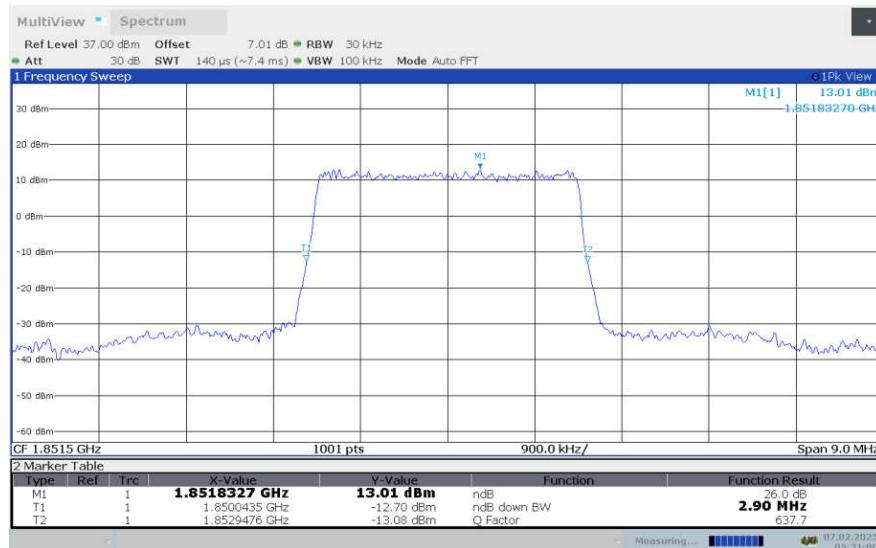
**LTE Band 2, 3MHz Bandwidth,LOW,16QAM (-26dBc OBW)**
