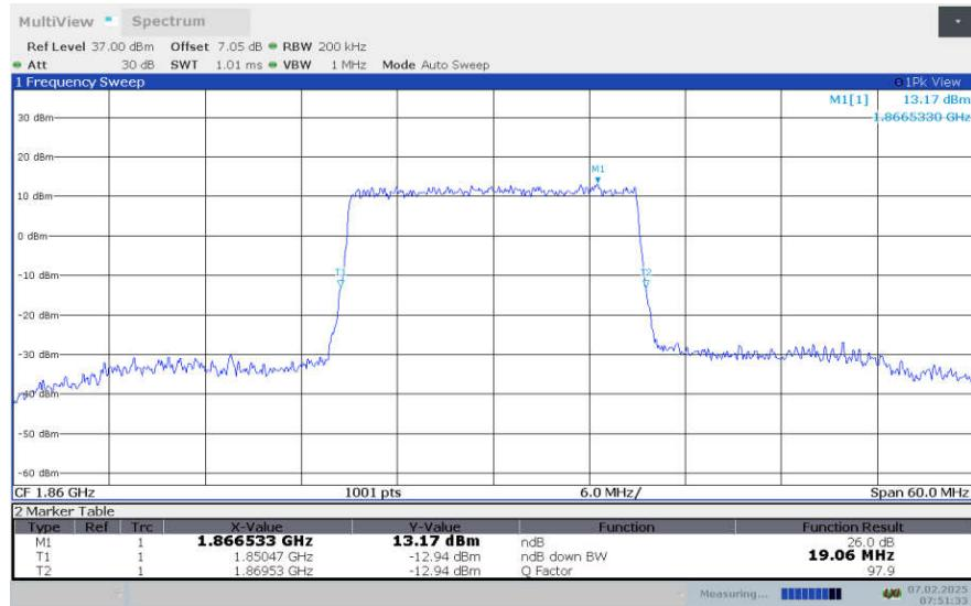
**LTE Band 2, 20MHz Bandwidth,LOW,16QAM (-26dBc OBW)**
