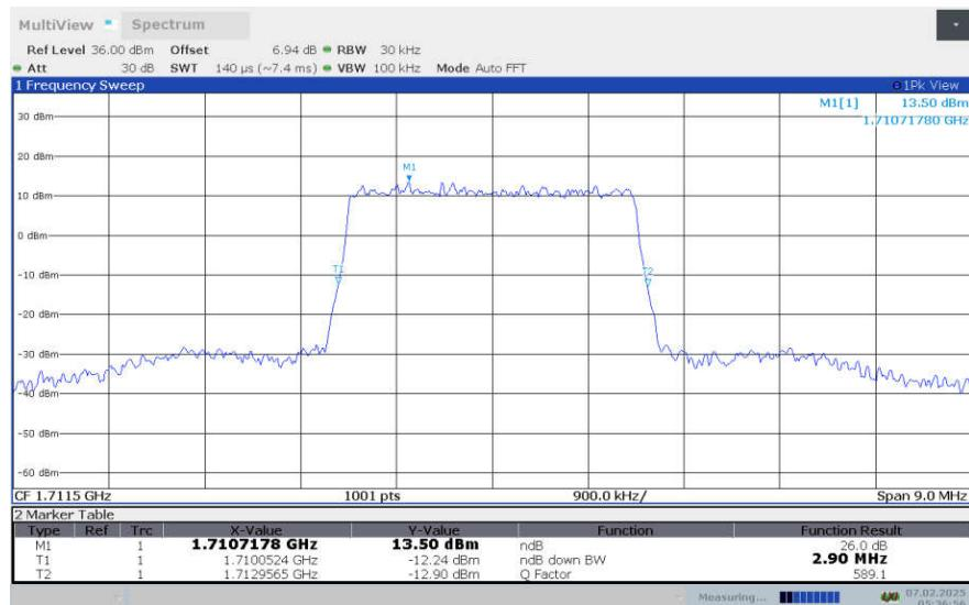
**LTE Band 4, 3MHz Bandwidth,LOW,64QAM (-26dBc OBW)**
