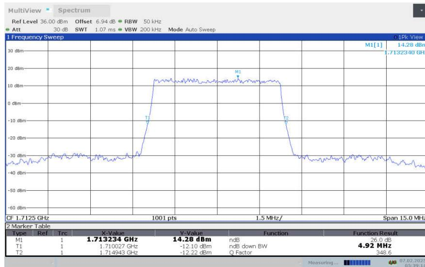
**LTE Band 4, 5MHz Bandwidth,LOW,16QAM (-26dBc OBW)**
