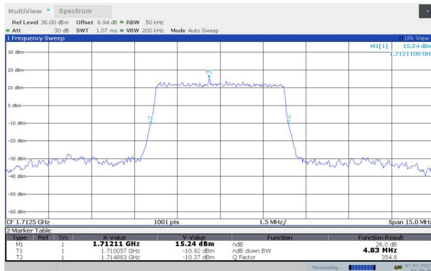
**LTE Band 4, 5MHz Bandwidth,LOW,64QAM (-26dBc OBW)**
