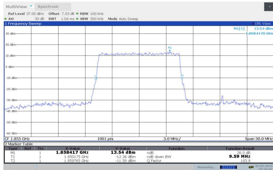
**LTE Band 2 , 10MHz Bandwidth,LOW,16QAM (-26dBc OBW)**
