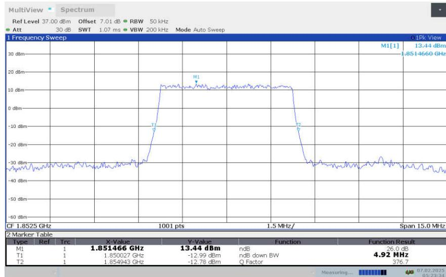
**LTE Band 2, 5MHz Bandwidth,LOW,16QAM (-26dBc OBW)**
