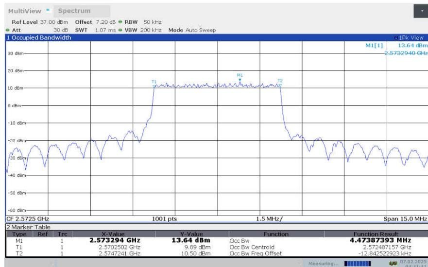
**LTE Band 38, 5MHz Bandwidth,LOW,64QAM (99% OBW)**
