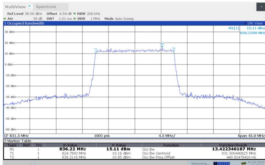
**LTE Band 26 , 15MHz Bandwidth,LOW,64QAM (99% OBW)**
