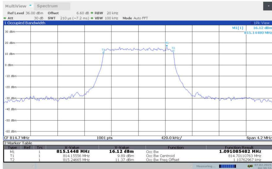
**LTE Band 26 , 1.4MHz Bandwidth,LOW,16QAM (99% OBW)**
