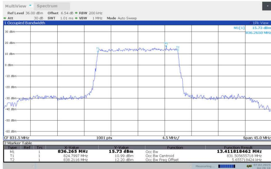
**LTE Band 26 , 15MHz Bandwidth,LOW,16QAM (99% OBW)**
