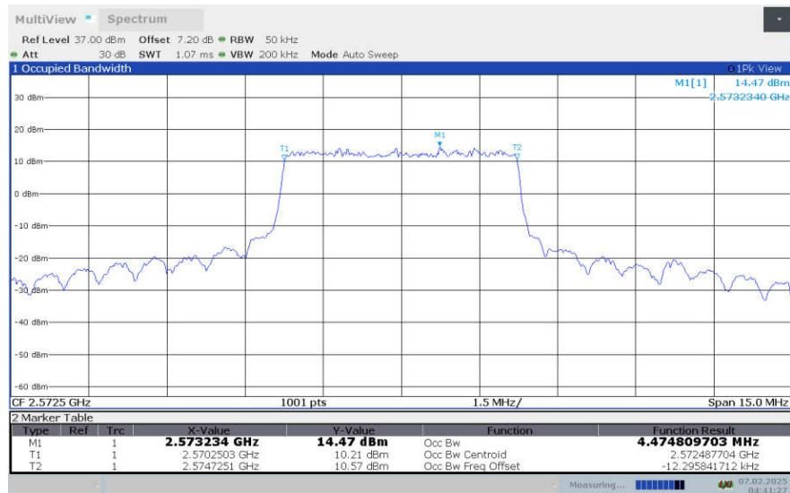
**LTE Band 38, 5MHz Bandwidth,LOW,16QAM (99% OBW)**
