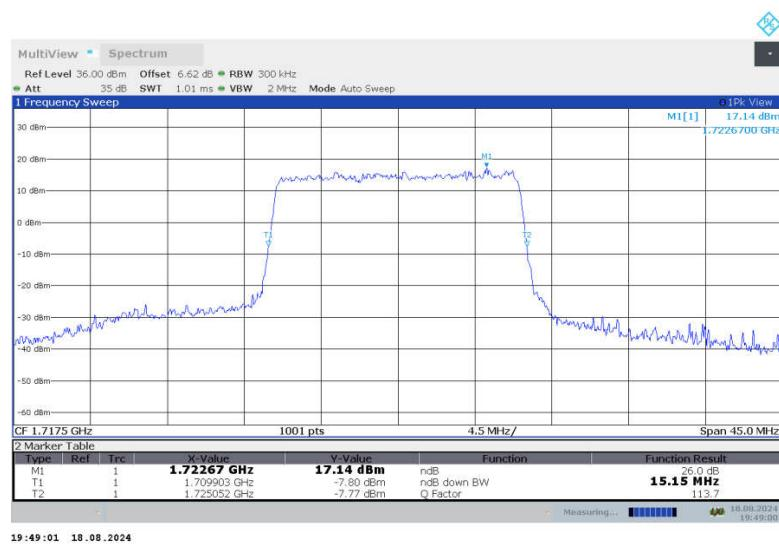
**n66,15MHz Bandwidth,DFT-s-QPSK (-26dBc BW)**
