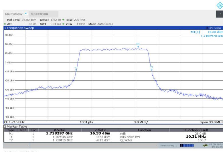
**n66,10MHz Bandwidth,DFT-s-QPSK (-26dBc BW)**
