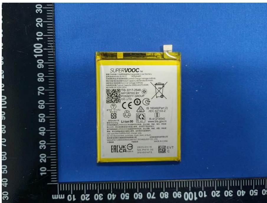
Battery Photo (REAR)
