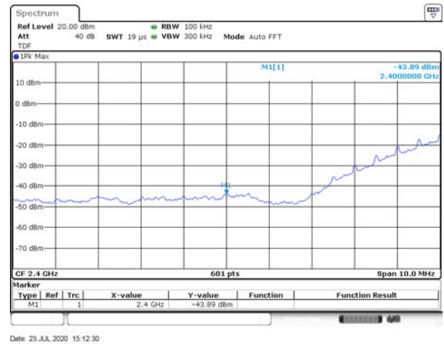
802.11b LOW CHANNEL, Reference level
