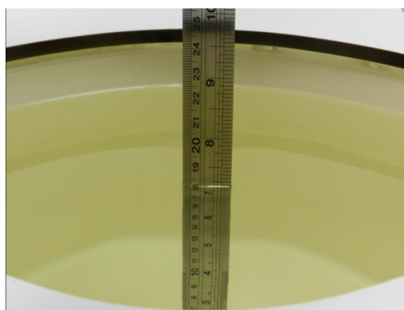
Fig 10.2 Photo of Liquid Height for Body SAR
