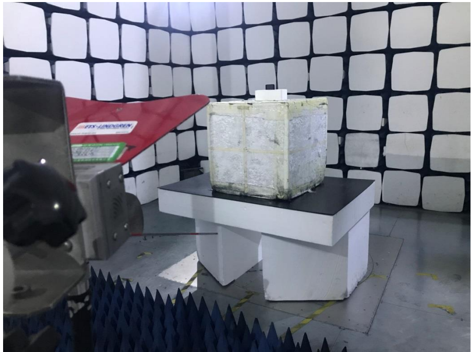
Radiation Emission Test Setup (1GHz to 18GHz)
