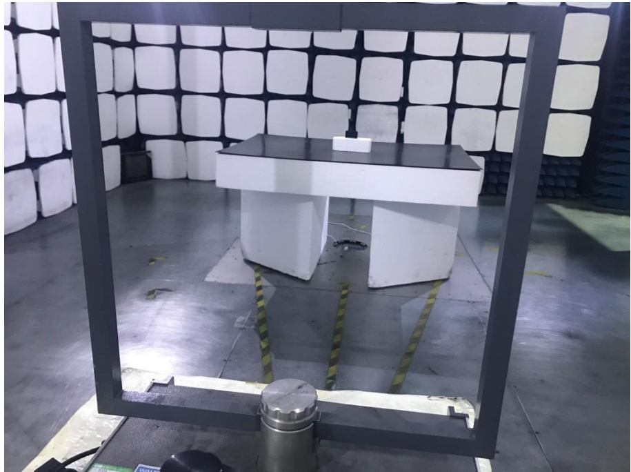
Radiation Emission Test Setup (Below 30MHz)
