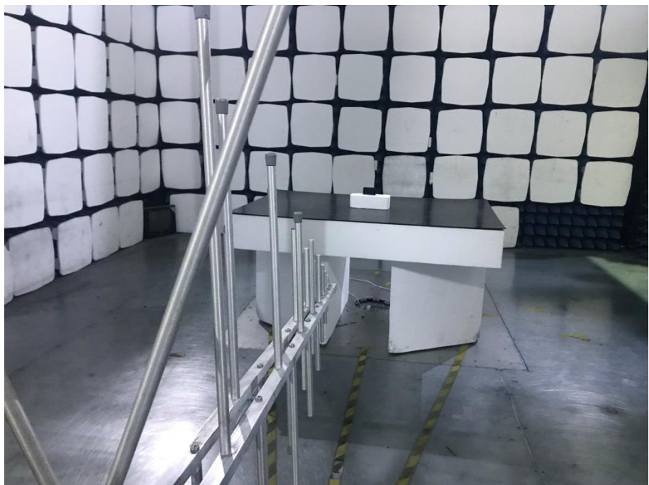
Radiation Emission Test Setup (30MHz to 1GHz)
