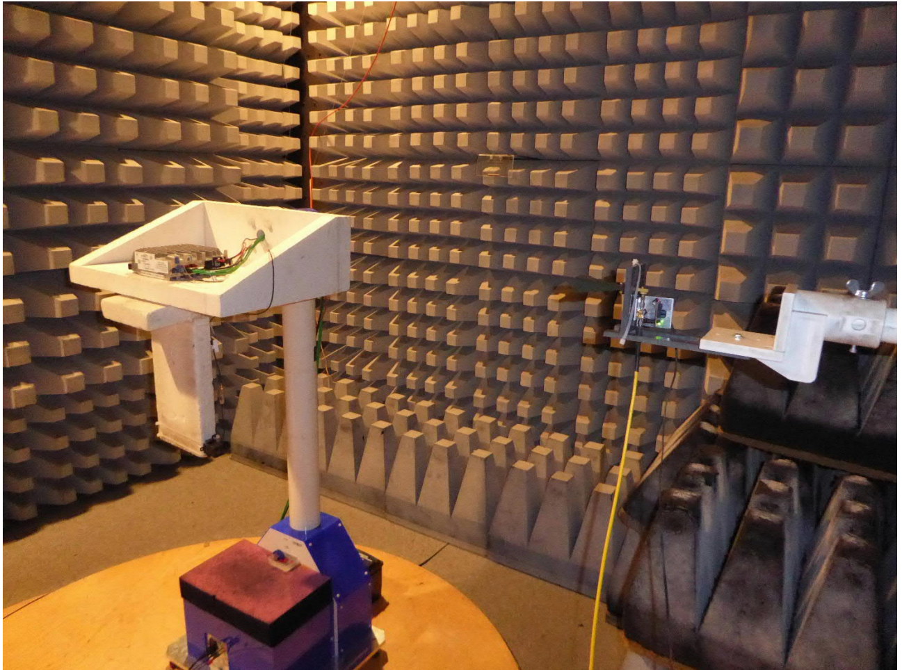
Test setup fully anechoic chamber (26.5 – 40 GHz)
