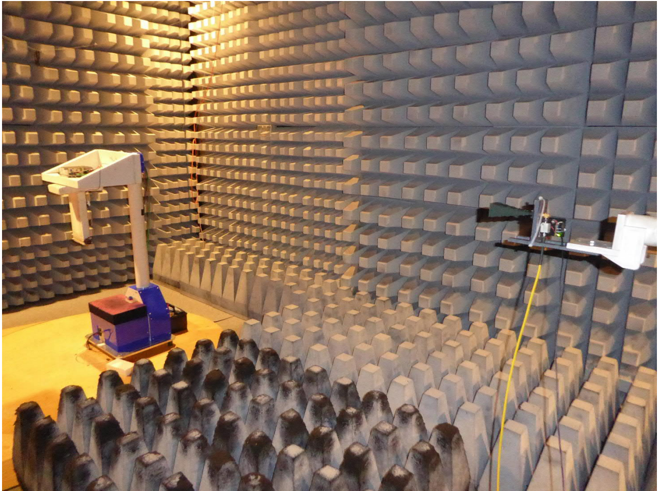
Test setup fully anechoic chamber (18 – 26.5 GHz)
