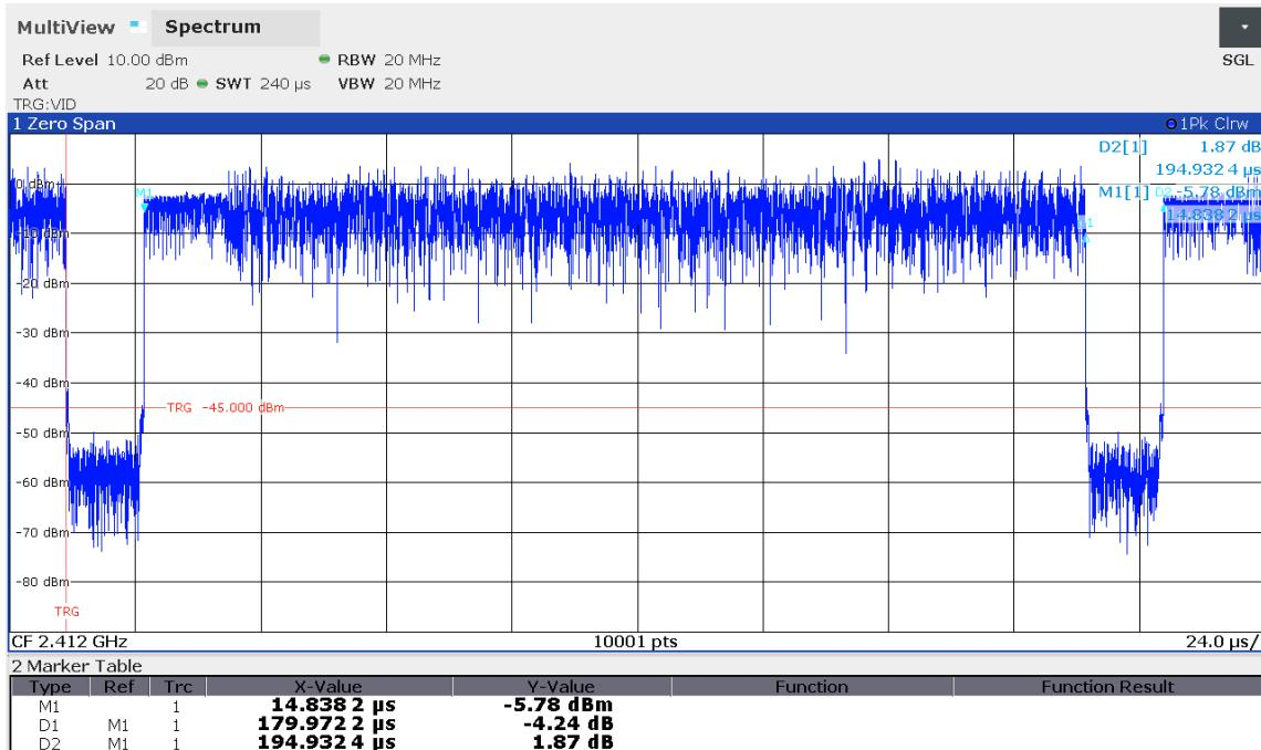
Only the duty cycle for 802.11b,g were tested, because these tests were repeated completely with MiMo activated. For all other tests, the duty cycle correction factors from the original reports OT-223-RWD-043 by LG Innotek Co., Ltd. were used.
