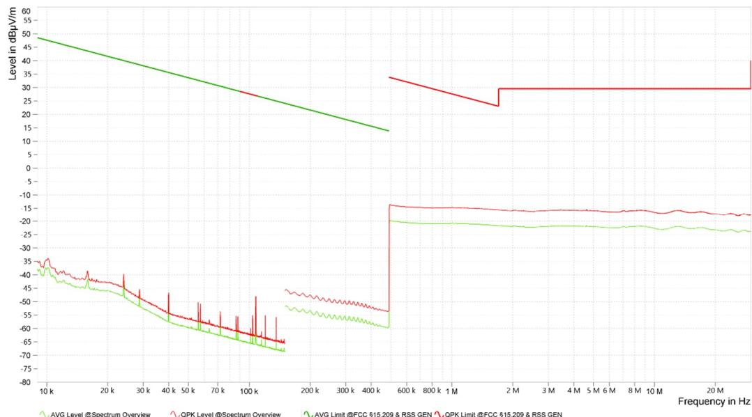
Remark: No emissions closer than 20 dB to the limit, so no final measurement will be carried out.
