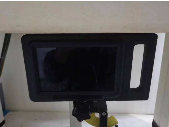
Fig-4.3 Top Side of EUT with 0 cm Gap (Body Mode)
