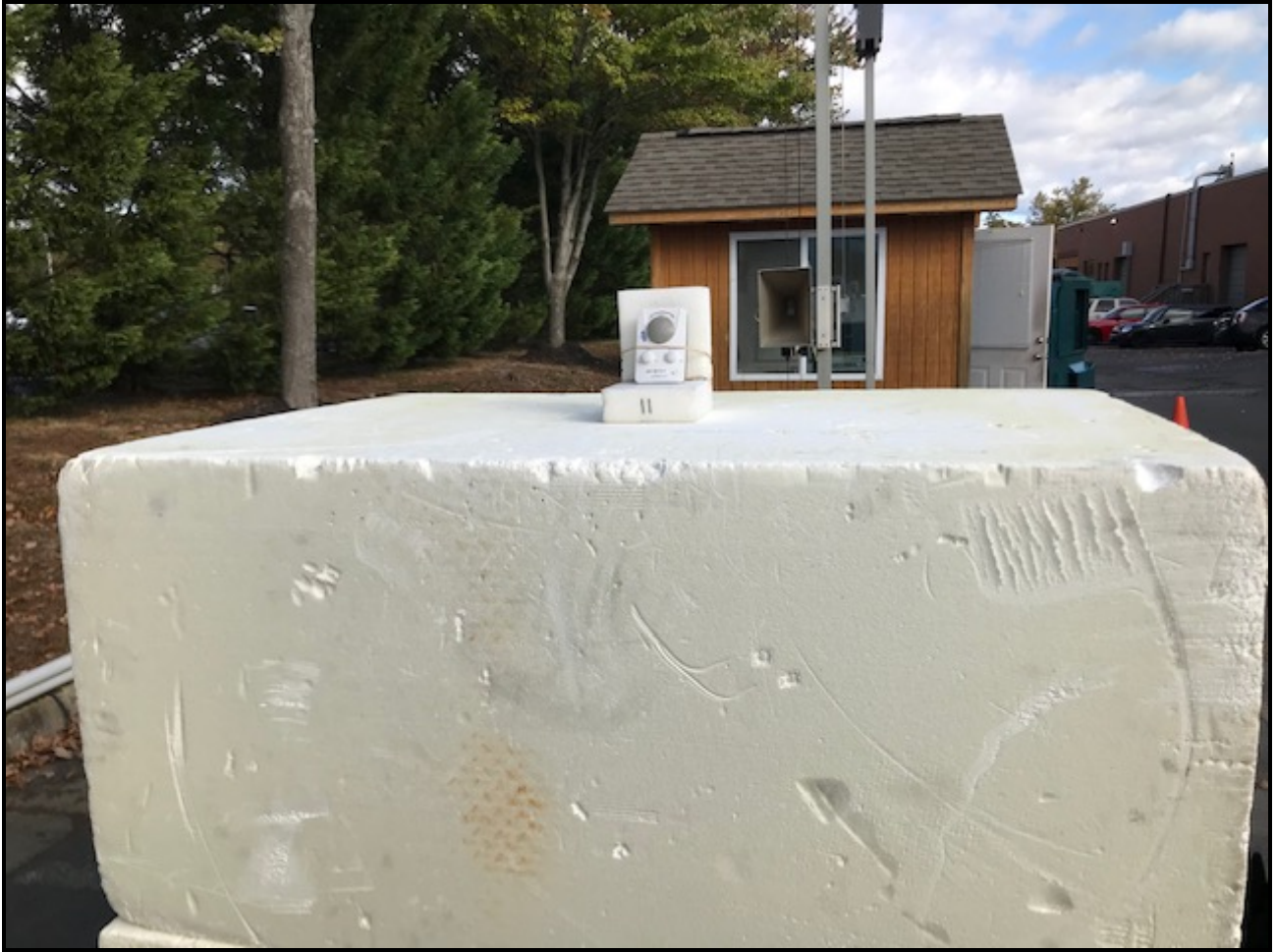
Photograph 3: Radiated Emissions Testing – Front View (Spurious Emissions, >1 GHz)
