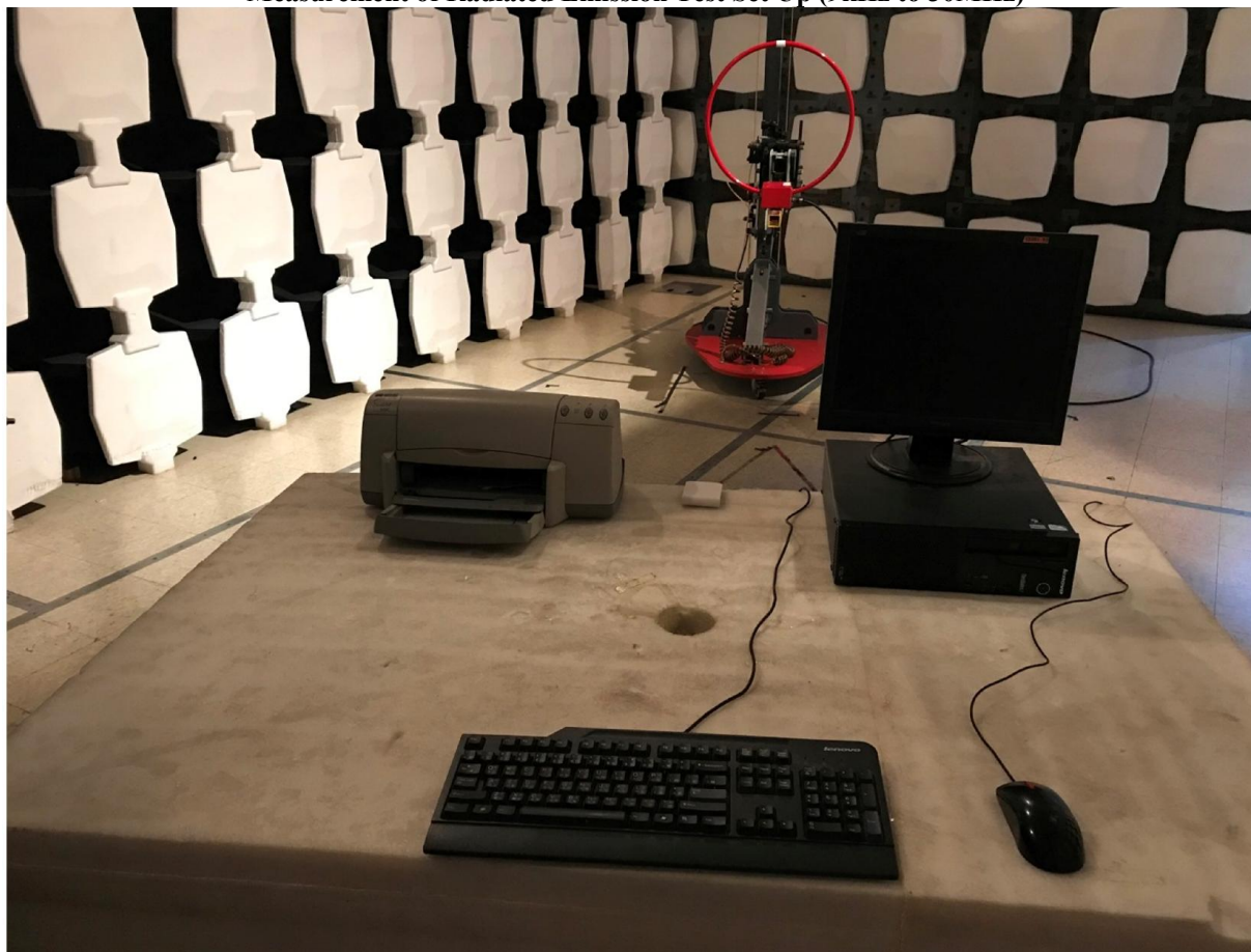
Measurement of Radiated Emission Test Set Up (9kHz to 30MHz)
