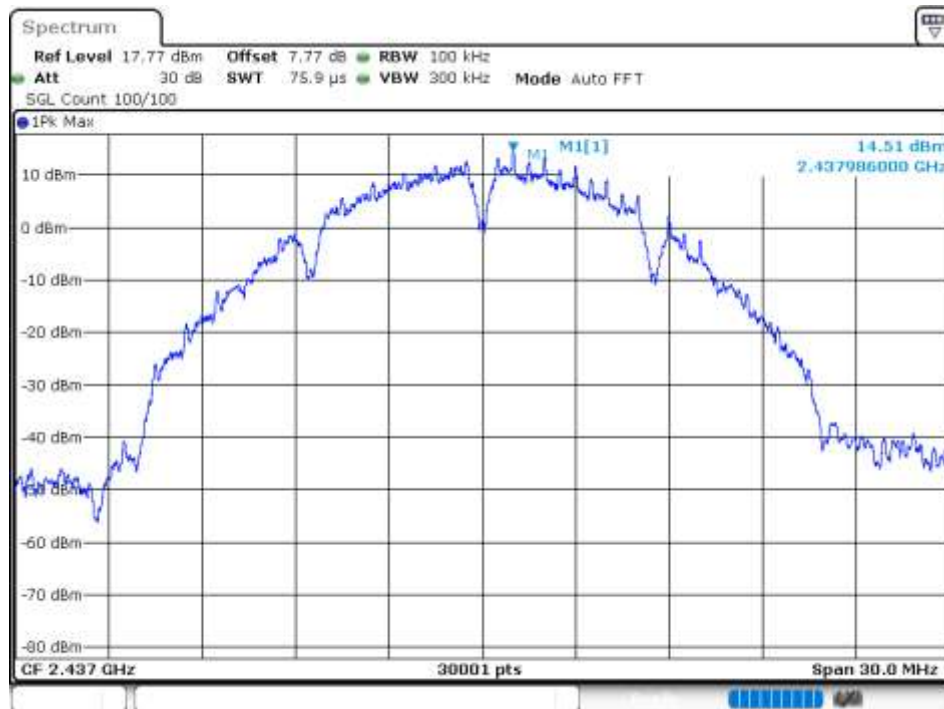
Tx. Spurious NVNT 802.11b 2437MHz Ant 2 Emission
