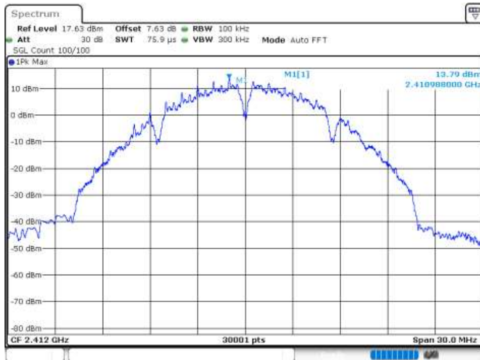
Tx. Spurious NVNT 802.11b 2412MHz Ant 2 Emission
