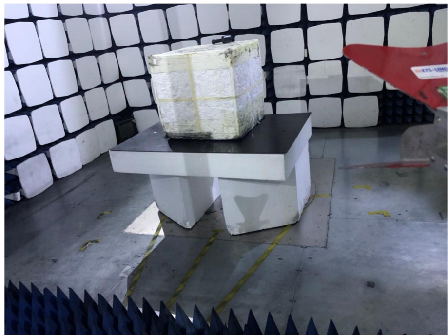
Radiation Emission Test Setup (1GHz to 18GHz)
