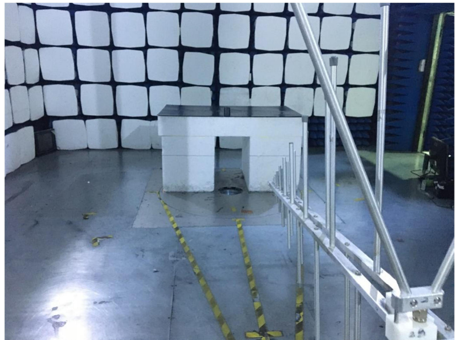
Radiation Emission Test Setup (30MHz to 1GHz)
