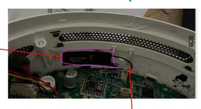
Assemble the coaxial line here
