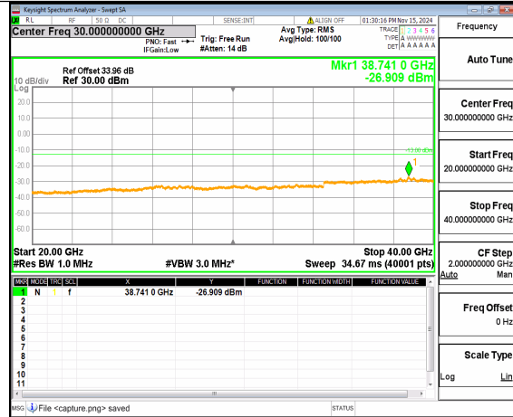
n77(3700-3980MHz) (20GHz-40GHz) 30M DFT-s-OFDM QPSK Inner_1RB_Right Mid
