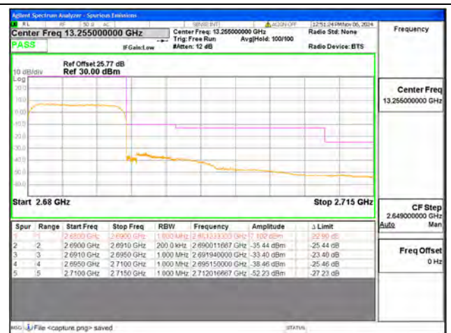
B41 / 10MHz / High CH / QPSK / FULL RB
