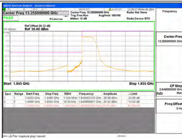
B25 / 3MHz / Low CH / QPSK / 1 RB
