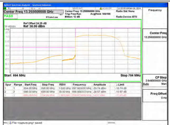
B12 / 3MHz / Low CH / QPSK / FULL RB
