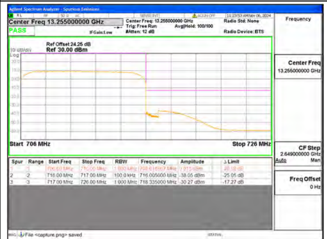
B12 / 10MHz / High CH / QPSK / FULL RB
