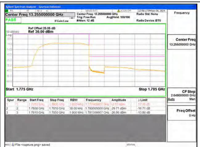
B66 / 3MHz / High CH / QPSK / FULL RB
