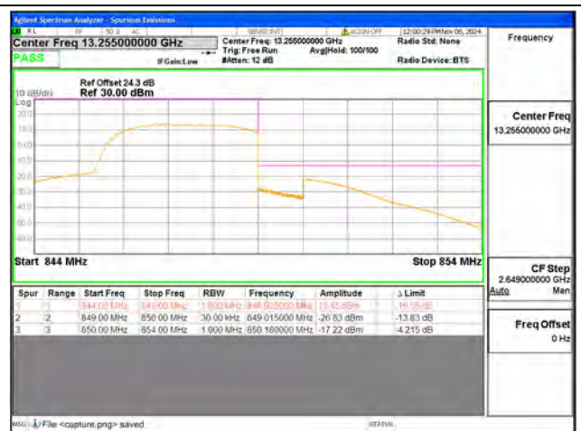
B26 / 3MHz / High CH / QPSK / FULL RB
