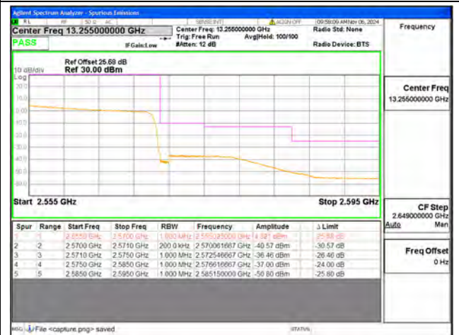
B7 / 20MHz / High CH / QPSK / FULL RB
