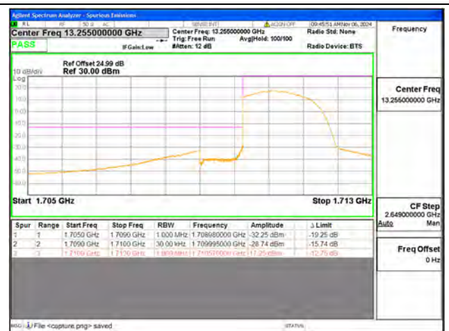
B4 / 1.4MHz / Low CH / QPSK / FULL RB
