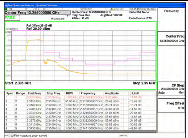
B30 / 5MHz / High CH / QPSK / FULL RB
