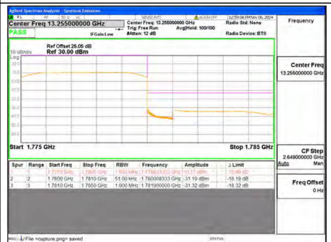
B66 / 5MHz / High CH / QPSK / FULL RB
