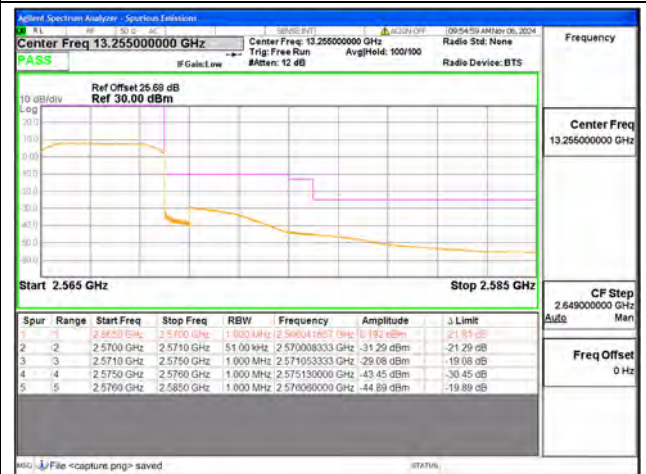
B7 / 5MHz / High CH / QPSK / FULL RB
