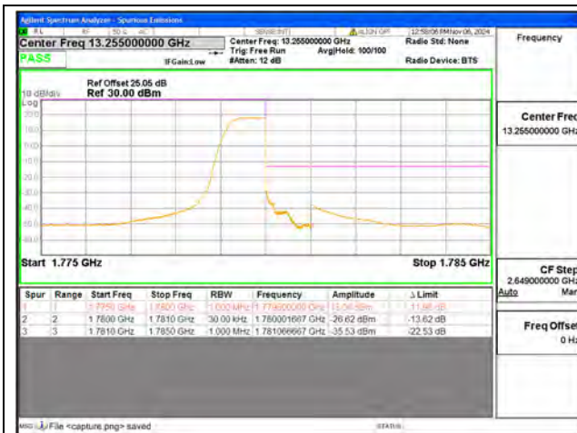
B66 / 3MHz / High CH / QPSK / 1 RB
