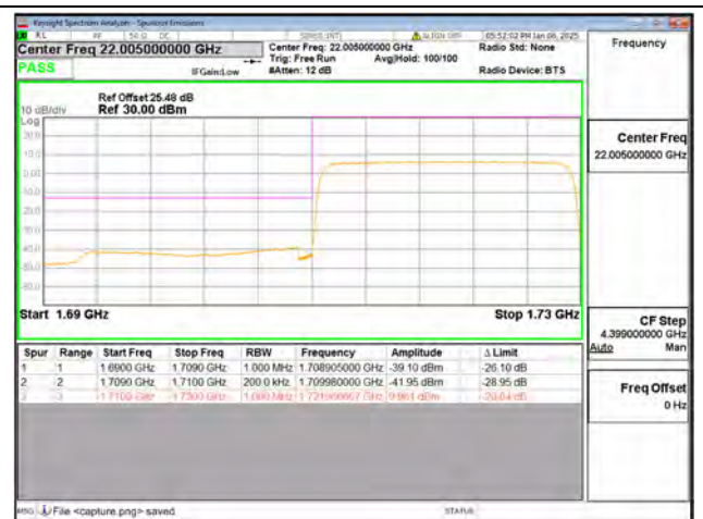
B4 / 20MHz / Low CH / QPSK / FULL RB
