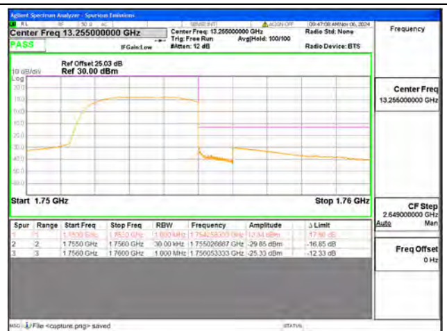
B4 / 3MHz / High CH / QPSK / FULL RB
