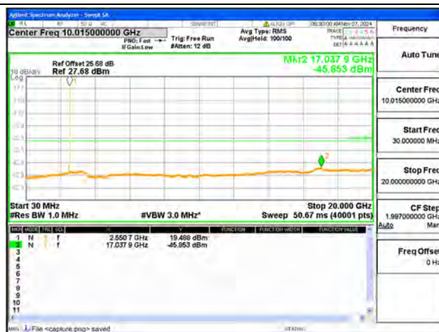
B7-30M-20G / 20MHz / High CH / QPSK
