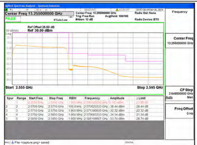
B7 / 15MHz / High CH / QPSK / FULL RB
