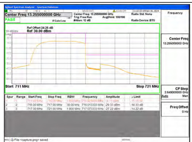
B12 / 3MHz / High CH / QPSK / FULL RB
