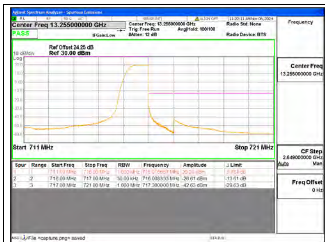
B12 / 3MHz / High CH / QPSK / 1 RB
