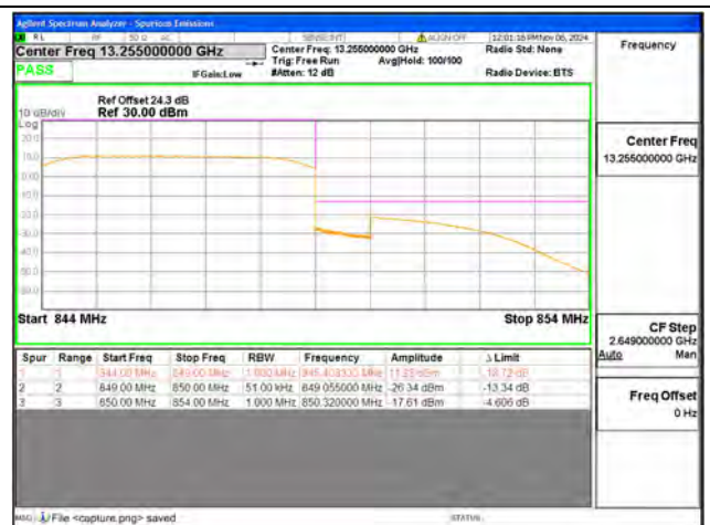
B26 / 5MHz / High CH / QPSK / FULL RB
