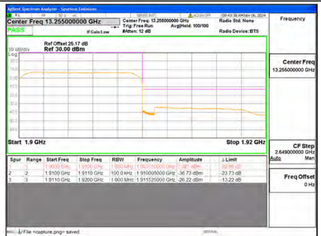
B2 / 10MHz / High CH / QPSK / FULL RB
