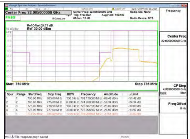
B13 / 5MHz / Low CH / QPSK / FULL RB
