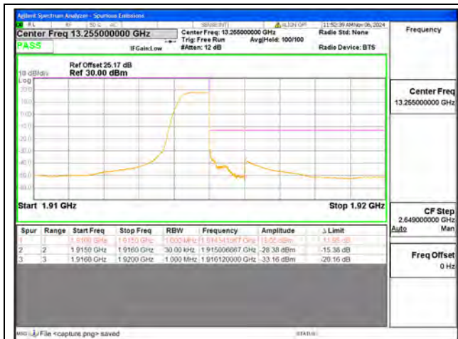
B25 / 3MHz / High CH / QPSK / 1 RB
