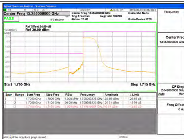
B4 / 3MHz / Low CH / QPSK / 1 RB
