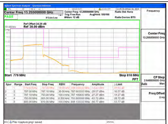
B13 / 5MHz / High CH / QPSK / FULL RB
