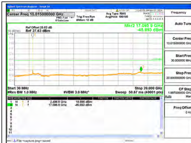
B41-30M-20G / 20MHz / Low CH / QPSK
