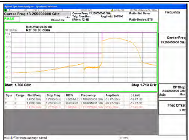
B66 / 1.4MHz / Low CH / QPSK / FULL RB
