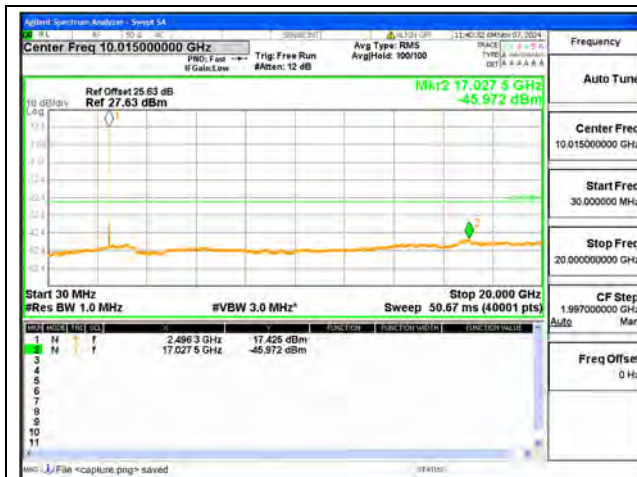
B41-30M-20G / 15MHz / Low CH / QPSK
