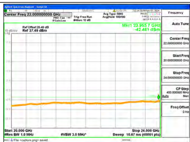
B30-20G-24G / 5MHz / High CH / QPSK
