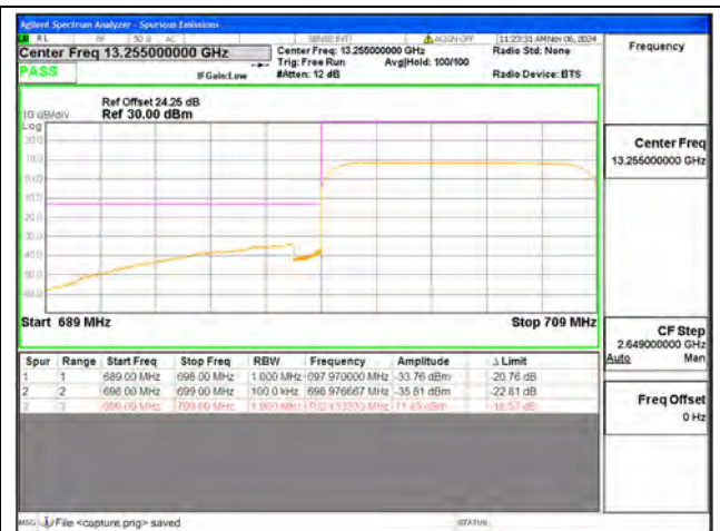
B12 / 10MHz / Low CH / QPSK / FULL RB
