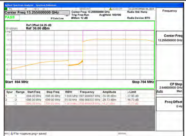
B12 / 5MHz / Low CH / QPSK / FULL RB
