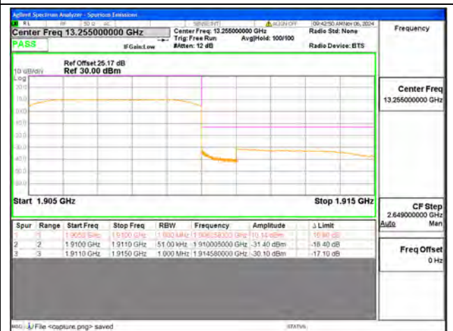
B2 / 5MHz / High CH / QPSK / FULL RB
