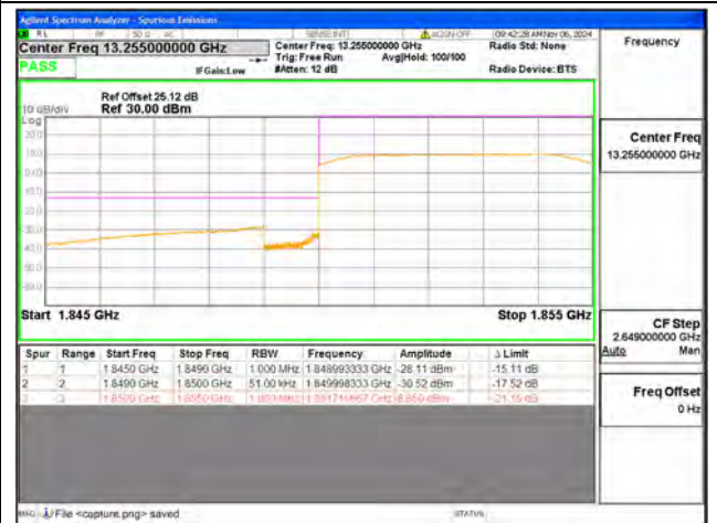
B2 / 5MHz / Low CH / QPSK / FULL RB
