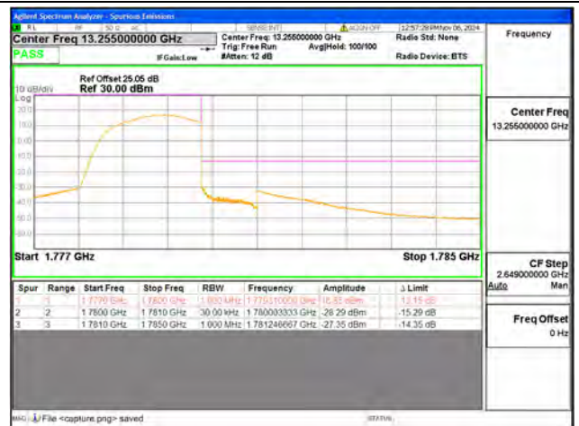
B66 / 1.4MHz / High CH / QPSK / FULL RB
