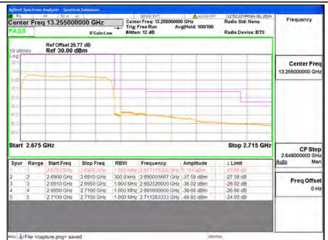
B41 / 15MHz / High CH / QPSK / FULL RB
