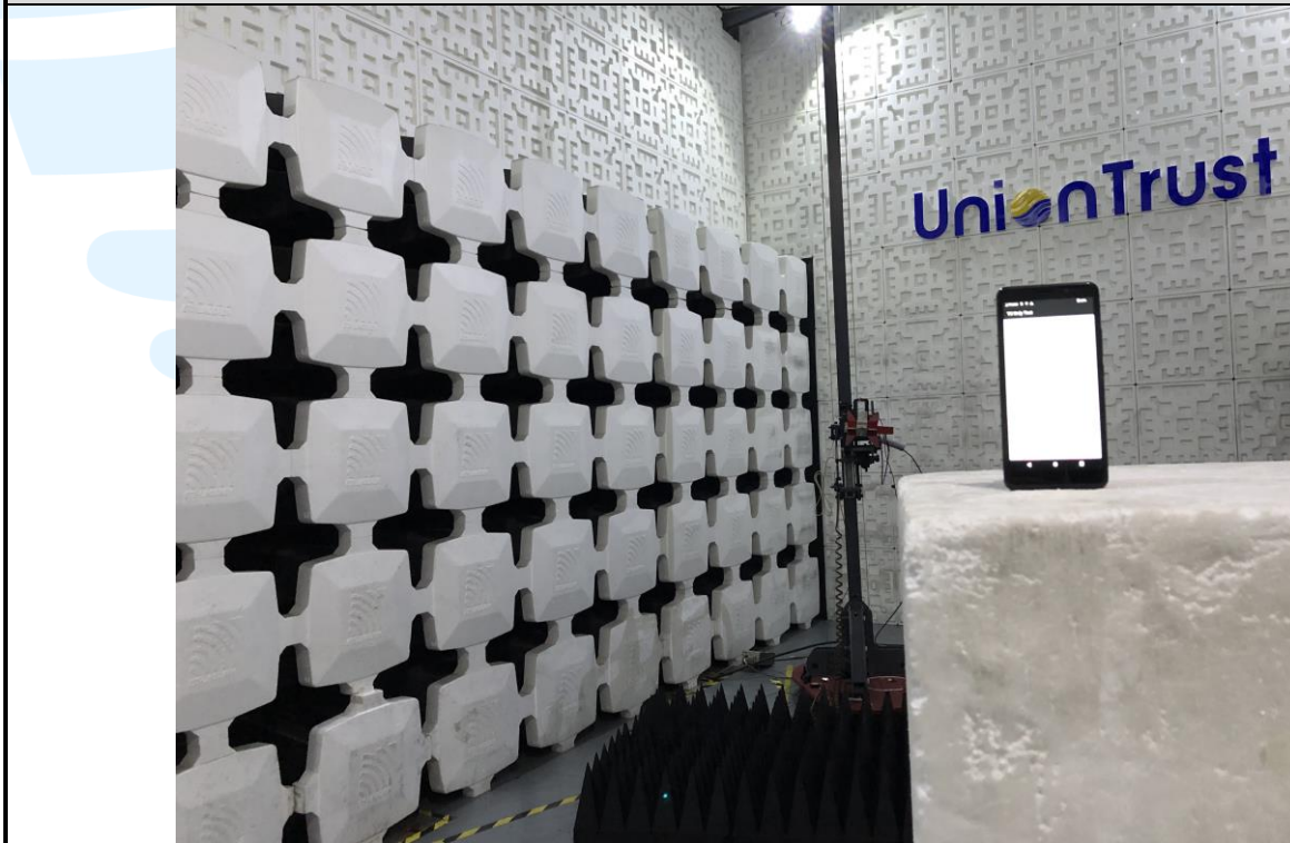
Radiated emission Test Setup (Above 1 GHz)
