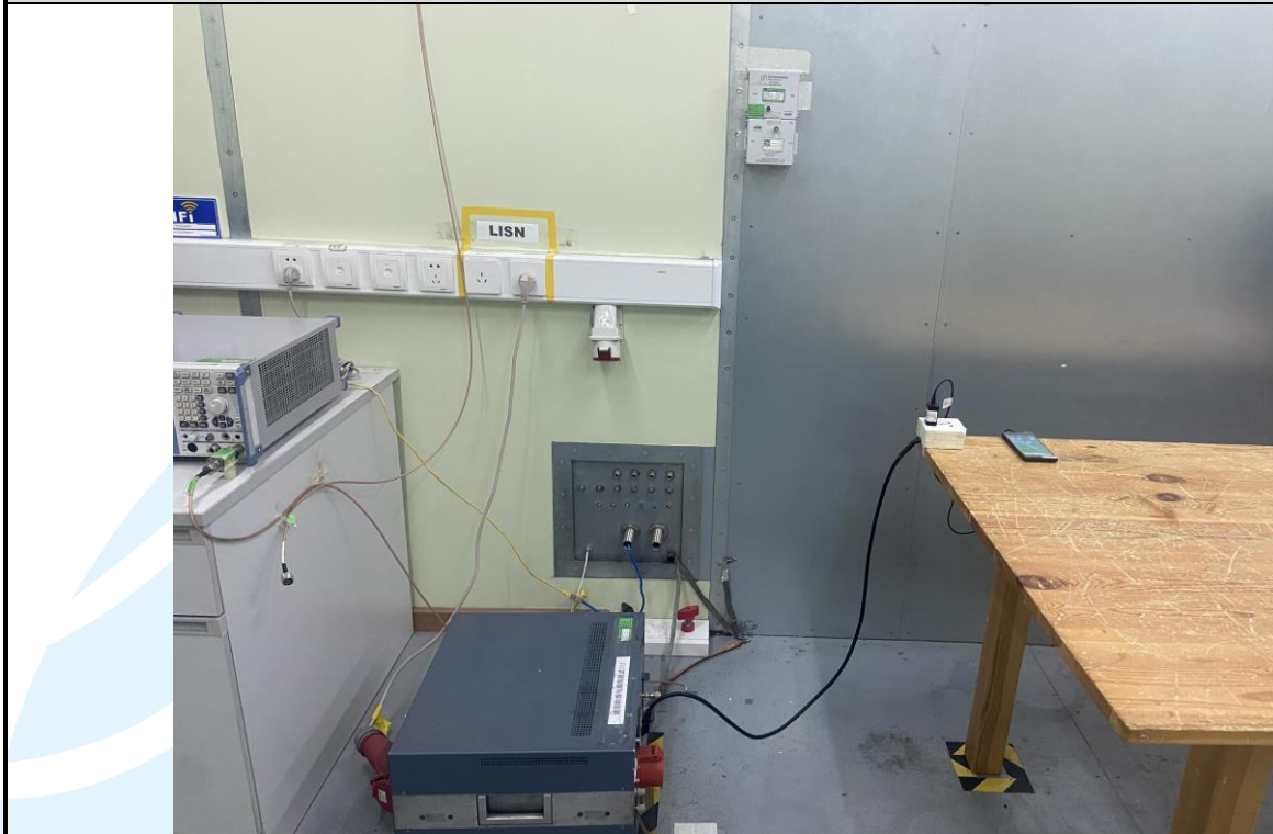
Conducted Emission Test Setup
