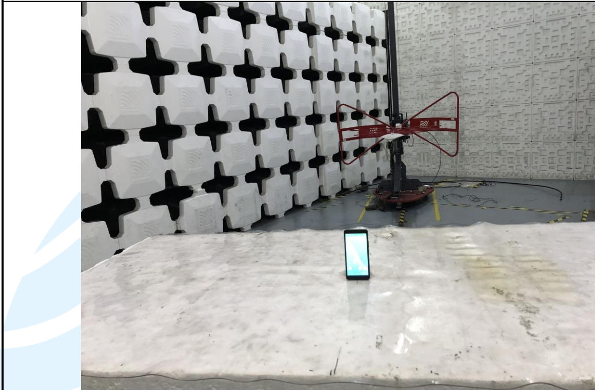
Radiated emission Test Setup (30 MHz~1 GHz)
