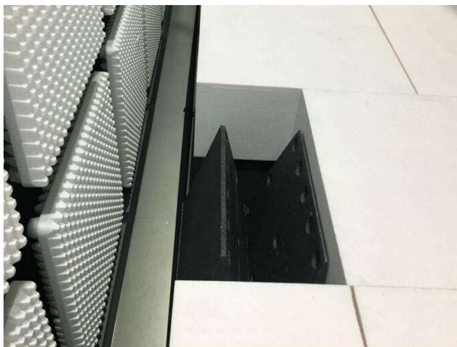
Radiated emission Test Setup-4(above 1GHz) There are absorbing materials under the ground.
