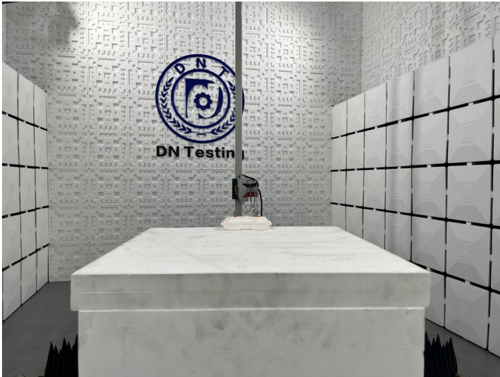
Radiated Emission Test View |(Above 1G)
