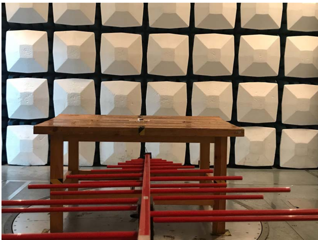
Radiated Emission Above 1GHz View
