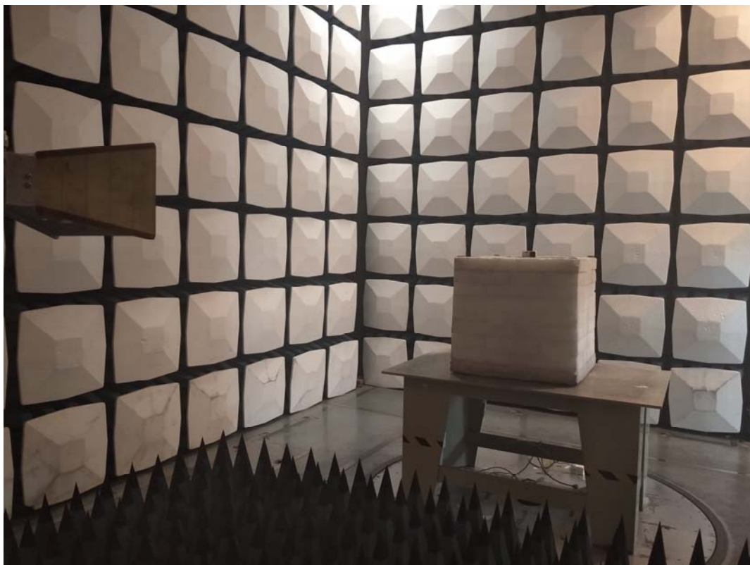
Radiated Emission Above 1GHz View
