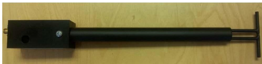
Figure 1 – MVG COMOSAR Validation Dipole
