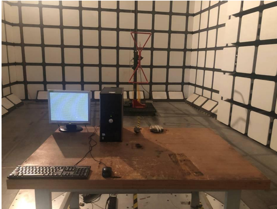
Radiated Emissions – Front View (Below 1 GHz)
