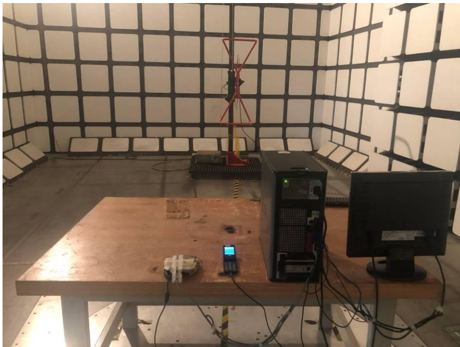
Radiated Emissions – Rear View (Below 1 GHz)
