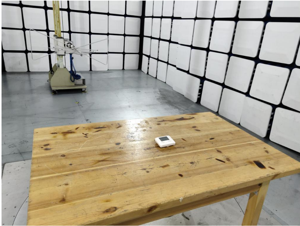
FCC ID: 2AUDN-STN715W Photo of Radiated Emission Measurement
