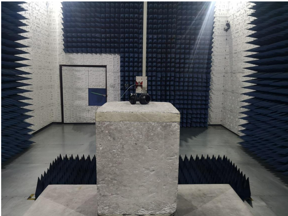
RADIATED EMISSION TEST SETUP ABOVE 1GHz
