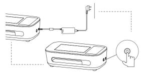
Connect the power cord to the adapter and socket. To ensure the normal operation of the device, please use 100-240volts AC power. Connect the adapter to the power interface of the device; Install the blade kit on the clamp to ensure it is fixed correctly. After connecting, press [PowerSwitch]to start the device.
