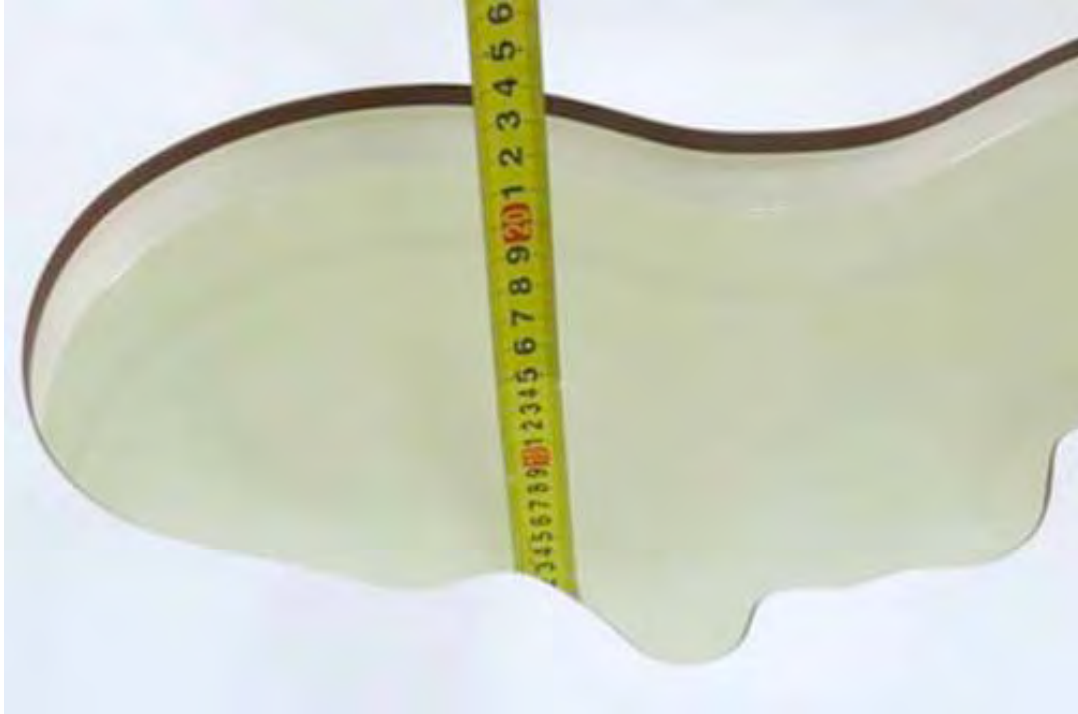
Picture 3: liquid depth in the head Phantom
