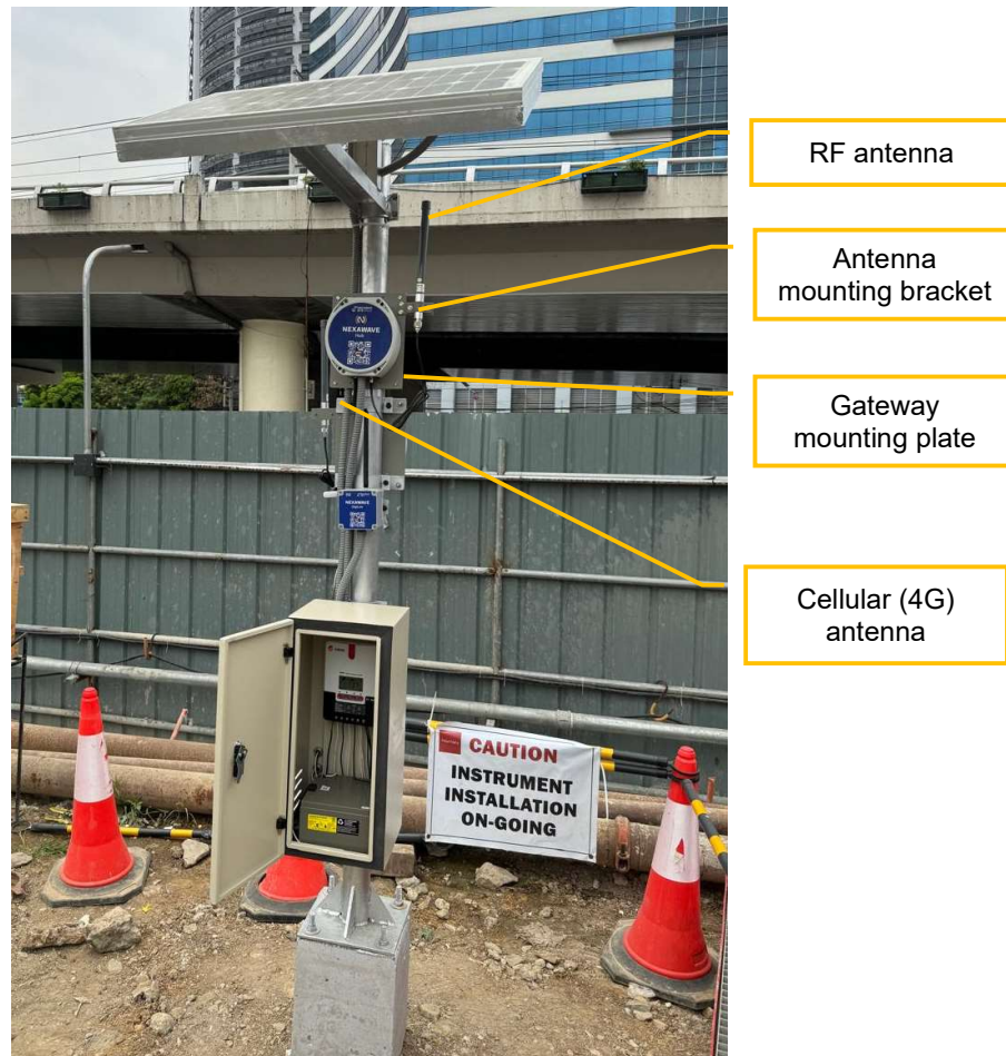
Figure 7-2 Gateway mounted on mast
