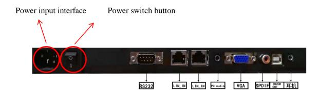
Please plug in the power cord. At this time, the indicator light on the front frame of the machine will light up, and the red color will indicate standby status.
