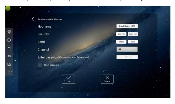
Wireless hotspots are available with 2.4G and 5G frequencies. Try to use 5G hotspots when transferring screens, which can improve transmission efficiency.
