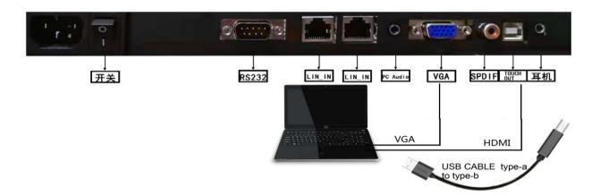
When the machine receives an HDMI or VGA signal from an external computer, the machine's touch control signals can be output from this "touch out" port, which the user can connect to the computer using a USB cable. After that, the user can operate the computer from the screen of the machine.
