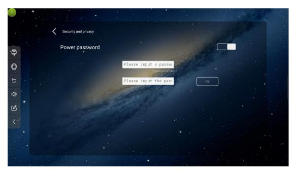
The power-on password is an 8-digit alphanumeric password. After booting and restarting, it will enter the power-on password interface first.
