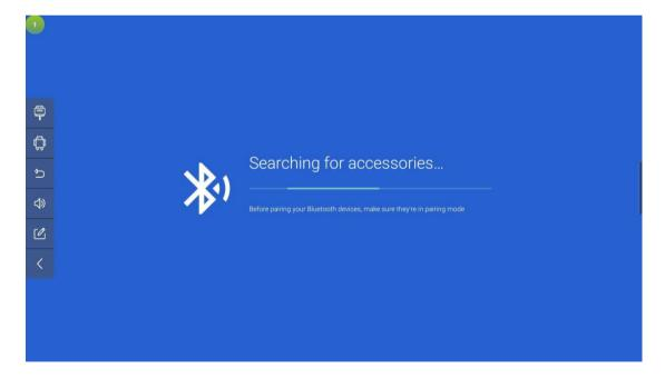
After searching for a Bluetooth device, click on the corresponding Bluetooth device name to link the Bluetooth device for audio playback.
