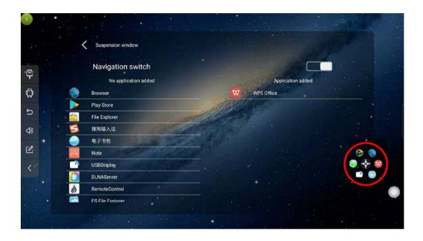
The left side can be added to the floating navigation app, the right side is the added navigation app, and up to 6 apps can be added.
