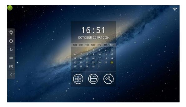
When booting, the machine will default to the system desktop as above. Some models with an OPS built-in computer will default to the OPS computer interface when the machine boots. At this point, you can directly operate the OPS computer. If you need to return to the main interface, you can return it by operating the sidebar shortcut menu.
