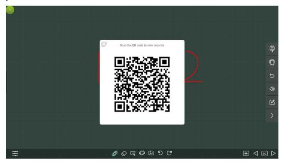
Internet options determine whether the QR code is a WAN link or a local hotspot link. If it is a local hotspot link, then the mobile phone must be connected to the hotspot emitted by the machine to scan and download. If it is a WAN link, the machine must be connected to the Internet, and the phone can be connected to the Internet (only WeChat is supported).
