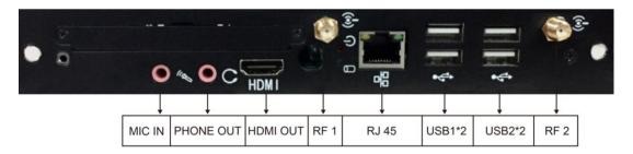
3. Bottom input port on the back of the machine
