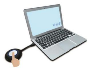
When the word "Shareable" appears on the lower right of the screen, the light of the screen will be always on, indicating that the screen connection is successful. (Some computer anti-virus programs will intercept the disc auto-run mode, you need to manually select the disc to run, open the screen program.)
