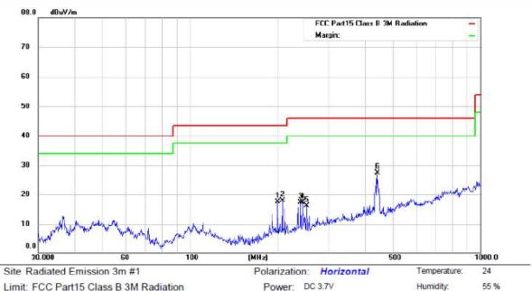
Limit: FCC Part15 Class B 3M Radiation Mode:TX (GFSK, 2480MHz)
