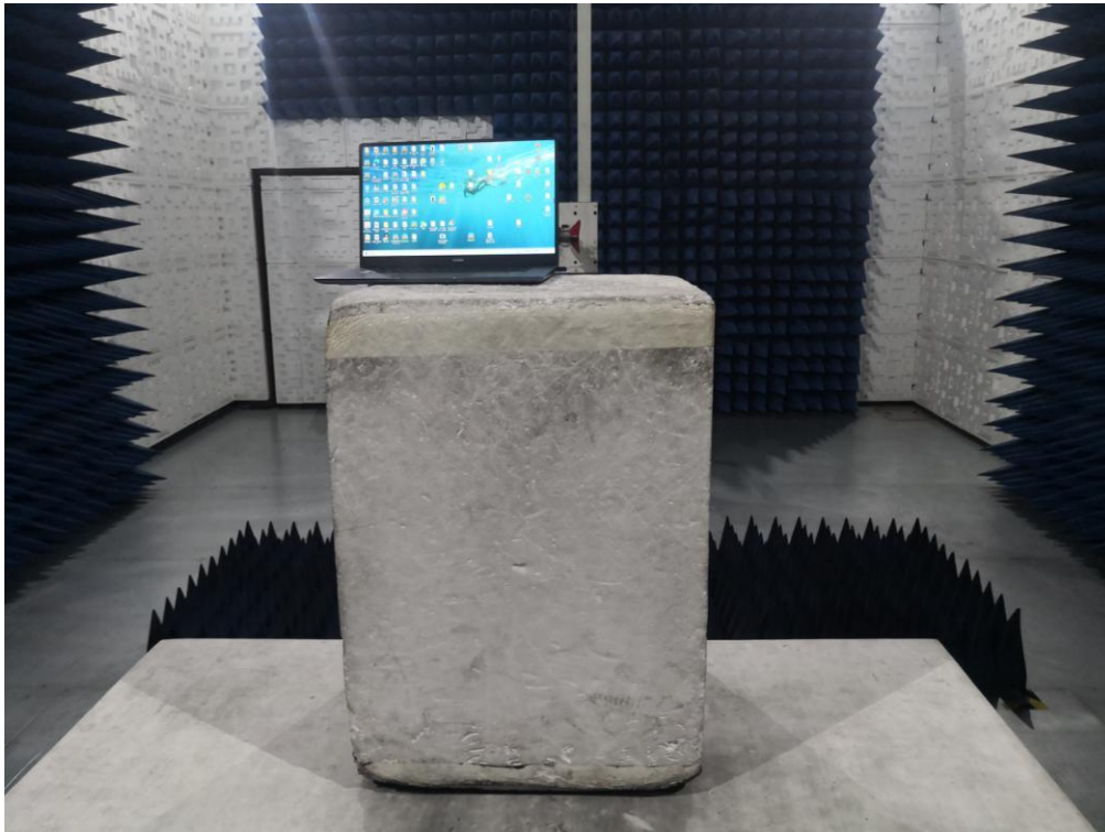
RADIATED EMISSION TEST SETUP ABOVE 1GHz
