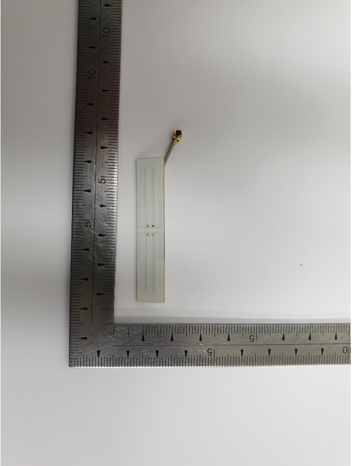
Antenna 2 (Additional) / PCB Antenna [Model name: AEi-2450/5500P-IPEX35]
