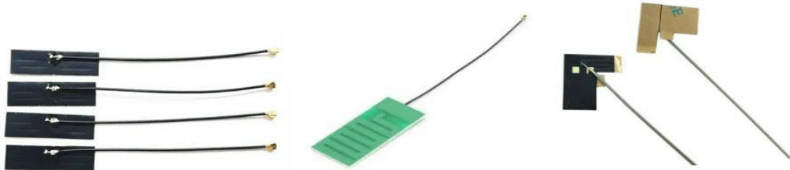
Figure 29 FPC antenna and PCB antenna
