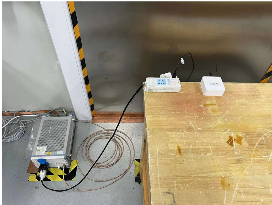
Test Set-up: Conducted emission 150KHz-30MHz
