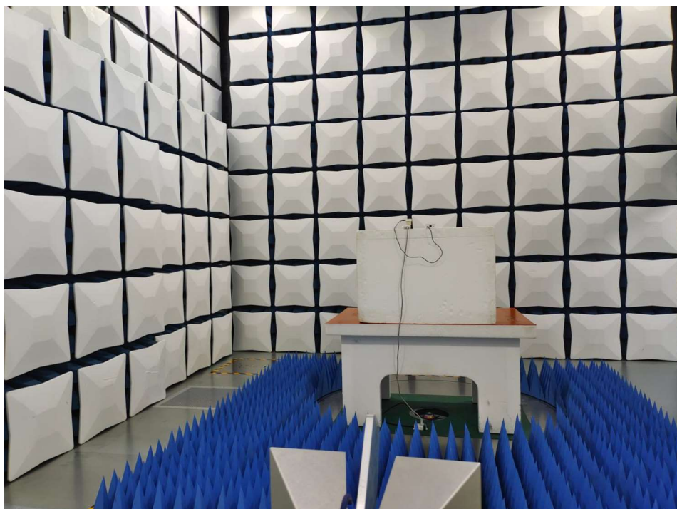
Test Set-up: Radiated spurious emission 1GHz-18GHz
