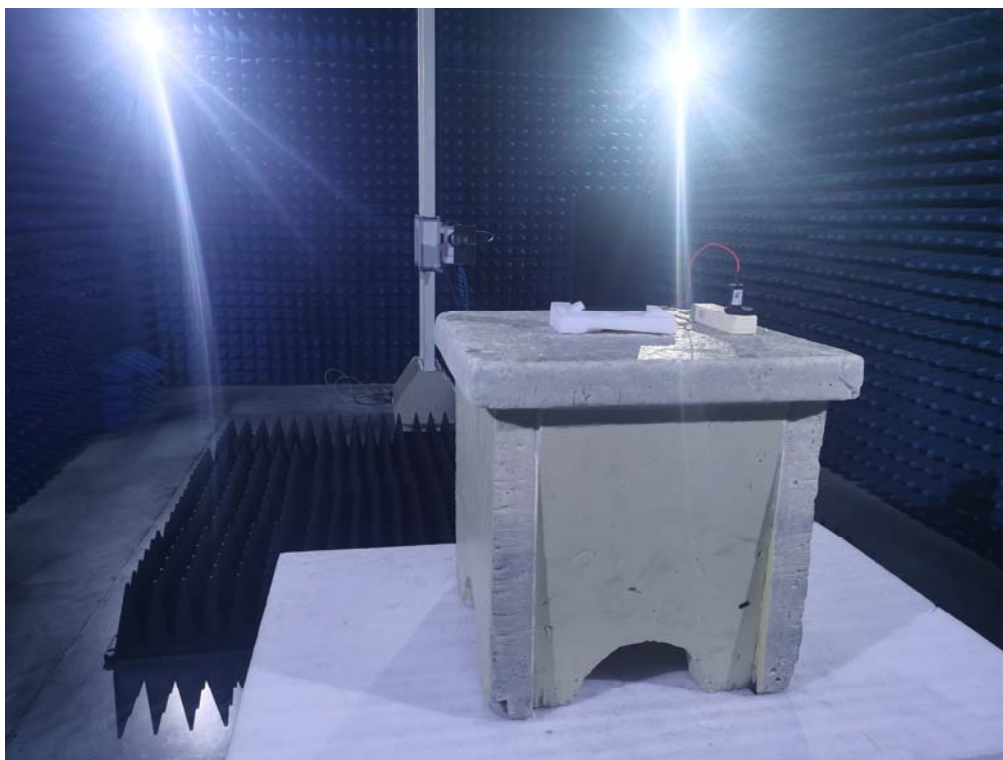
Photo of Radiated Emission Measurement (Above 1G)
