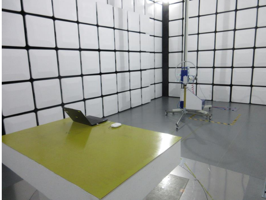
RADIATED RF MEASUREMENT SETUP (9kHz ~ 30 MHz)
