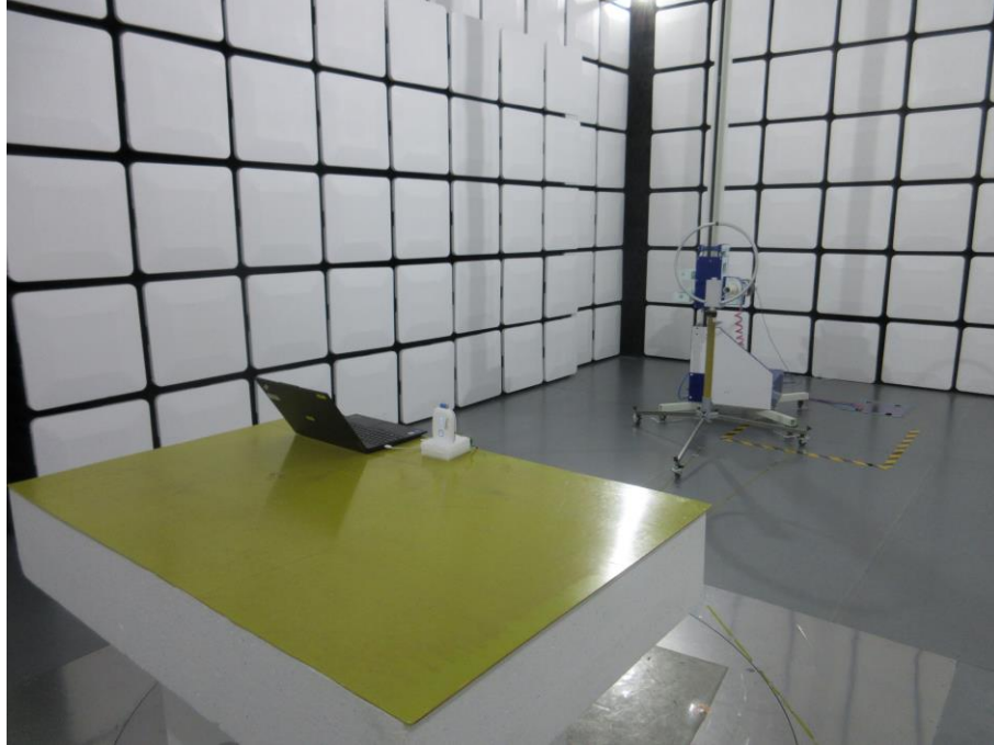
RADIATED RF MEASUREMENT SETUP (9kHz ~ 30 MHz)
