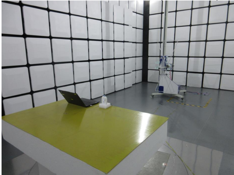
RADIATED RF MEASUREMENT SETUP (30MHz ~ 1 GHz)
